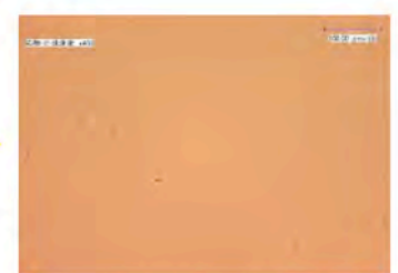
溶剤浸漬後 The resin and patterns are washed away
